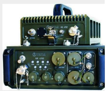
core for building of higher organizational levels in mobile tactical networks in NATO IV frequency band. Time continuous full duplex transmission capacity up to 320 Mbps is ensured by Frequency Division Duplex (FDD). Ethernet 10/100/1000 BASE-T and E1 (2048 kbps) are standard interfaces. Local control is over PC and IP management is over webserver or SNMP.
