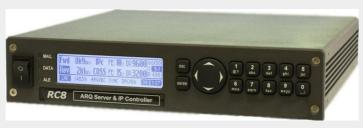
When used with the RM8 Software Defined Modem and external link encryptor, the RC8 provides robust, secure voice, data and position communication capability over HI links even in severely degraded channels conditions. This fully integrated, qualified system ensures optimal performance and functionality including voice, position transfer, Email, messaging, ACP 127 chat and IP data
