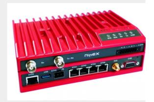
RipEX is a radio modem platform renowned for overall data throughput in any real-time environment. RipEX radio modems are native IP devices, Software Defined with Linux OS that have been designed with attentior to detail, performance and quality. All relevant state-of-the-art concepts have been carefully implemented.
